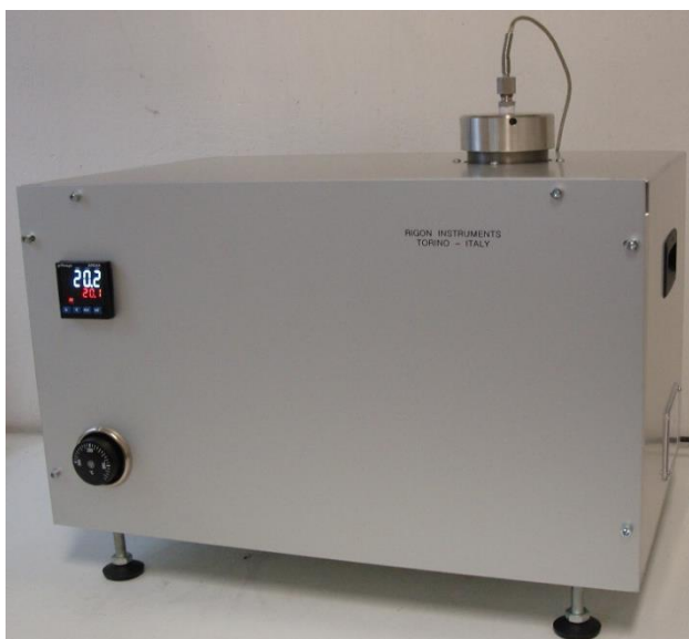
Heating system suitable for BOM
