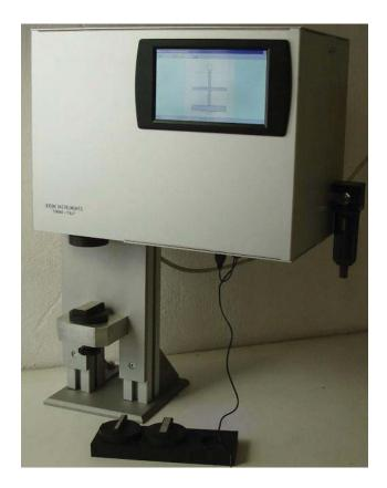
Interchangeable jaws automatically detected, allow adjustment within a large pressure and force margin. Thanks to the stable parallel guides of the moving jaws, high precision values are achieved even when the test piece is clamped not aligned. The pneumatic cylinder presses against the jaw holder via a compensation coupling. The fixed jaw is placed in a ball cup which has its center exactly at the surface of the jaw. With this, it is ensured that both jaws are always in a parallel position.
