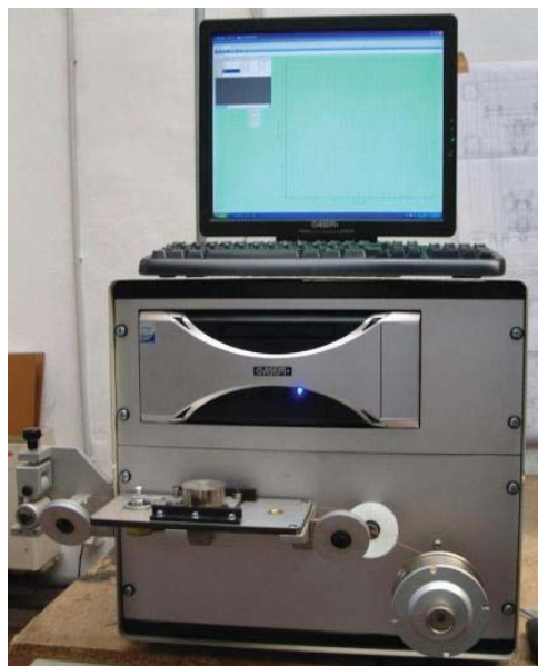
model SST (DIN 46453, IEC60851-3.B3)
